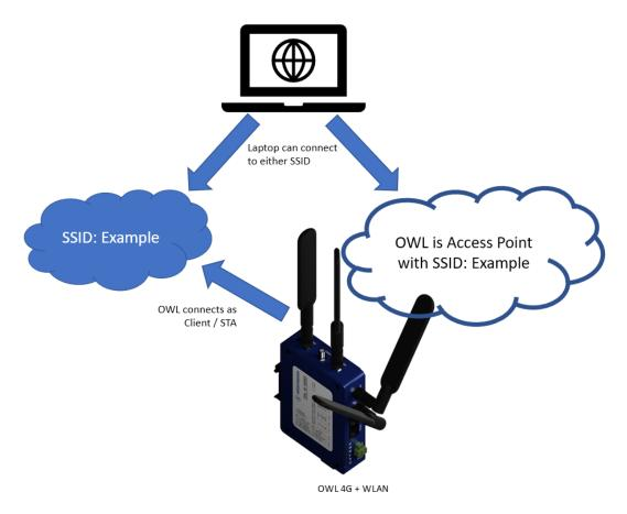
Some OWL variants support WLAN and can be configured to use both WLAN Cient and Access Point functionality at the same time.
