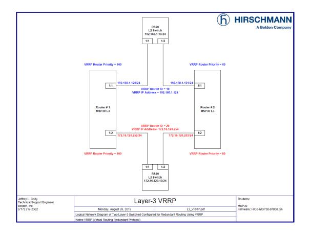
After having the basic routing functions configured and tested on the routers shown above, we will configure Router # 1 to function as the "Master" and Router # 2 to function as the "Backup" VRRP Routers for both the 192.168.1.0/24 and 172.16.12.0/24 networks.
