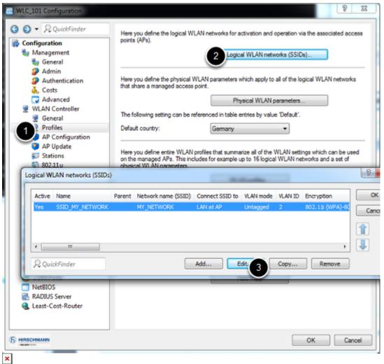
Configuration > WLAN Controller > Profiles > Logical WLAN networks (SSIDs) Select the Logical network you want to apply the RADIUS profile to (in our example ""SSID\_MY\_NETWORK"") Select Edit
