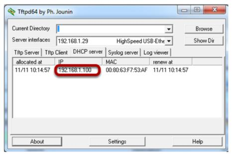
At the next DHCP request from the device, your DHCP server will automatically attribute to teh device an IP address from the defined pool of addresses.
