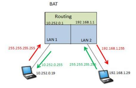
Redirect specific IP broadcast (depending on the UDP port) from IP NET 1 to IP NET 2 and vice versa :
