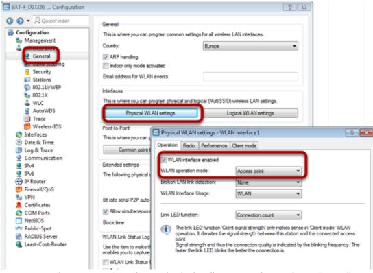
Use Access-Point as WLAN operation mode. Optionally you can choose alternative Radio settings etc.
