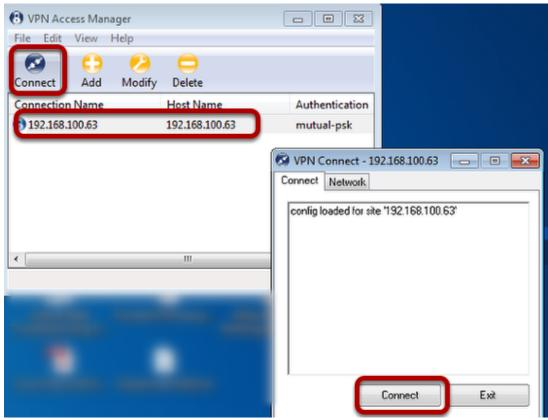
Mark the new created Vpn and press "Connect". A new window will open. Press "Connect".
