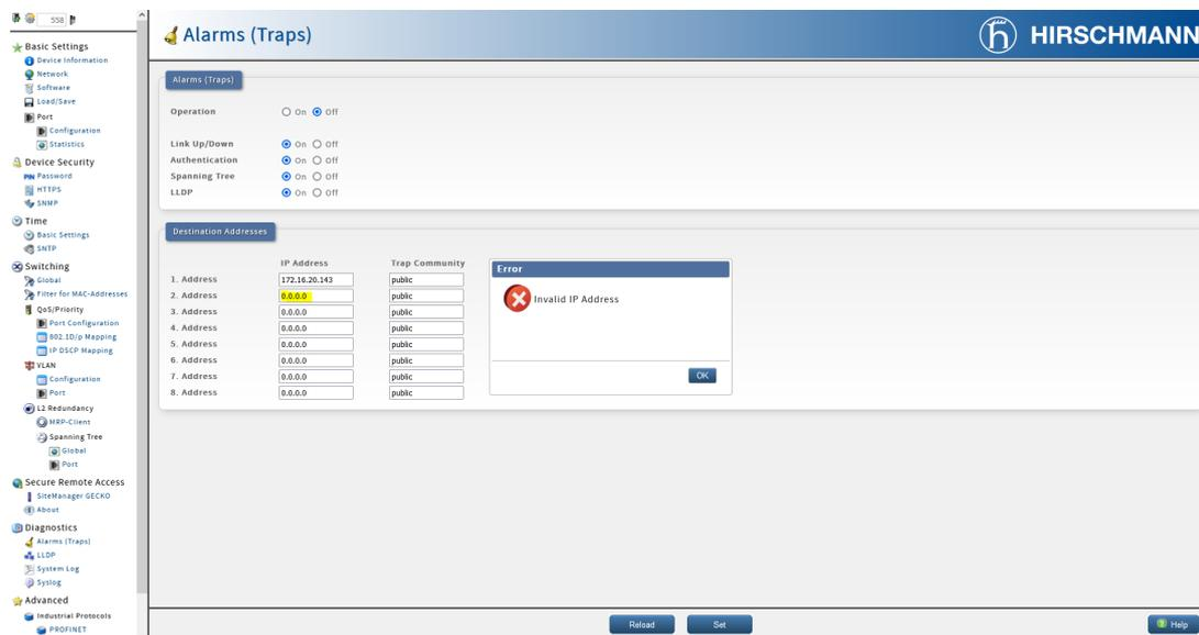
The screenshot shows the 'Alarms (Traps)' configuration page in the Hirschmann GECKO web interface. The page is divided into two main sections: 'Alarms (Traps)' and 'Destination Addresses'.
