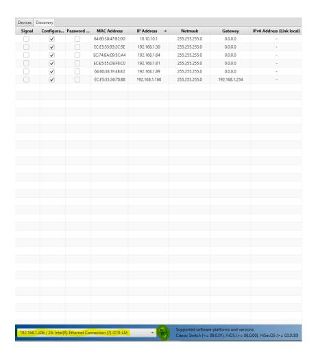
2. Double click on the device in the list and assign an IP address and click ok
