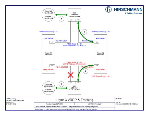
In the diagram above, if we have the same failure of the link between Router # 1 and the L2 switch in the 172 network, and Interface and Ping Tracking is properly configured, we can overcome the previous failure scenario by demoting the VRRP priority on Router # 1 if it senses a failure of the link on port 1/2 by lowering the VRRP priority to 70 for the VRRP router ID 10 on the 192 network.
