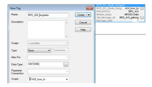
19. Click on the "Get\_Message\_all" config box and set the service code, class, Instance, and attribute to 1. Also set the Source element to the "msgdata[0] tag" created in a previous step. The "source length" is set to 2 and the "Destination element" is the msgdata[2]
