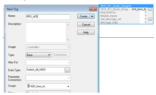
14. For the Module\_inputs select the I.Data from the switch created in previous step
