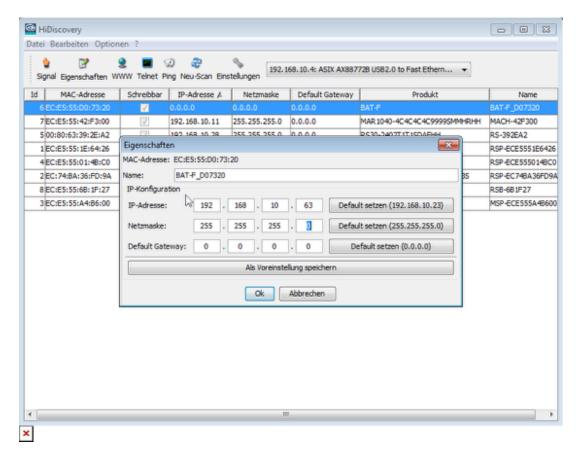
Use HiDiscovery to assign a IP-address to the BAT. The PC is locally connected.
