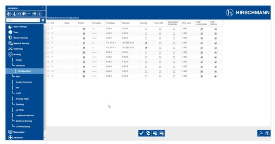
This completes the configuration steps required to configure Port-Based (Physical) Router Interfaces for Ports 1/4 and 1/5.
