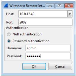
Give the IP address of the BAT, the RPCap port relevant username and password to access the device then clic ok
