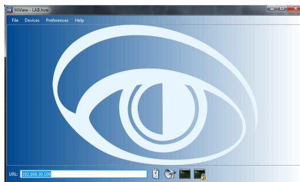
Enter the managed devices IP address into the URL box as shown, and hit "Enter" to proceed to the login screen
