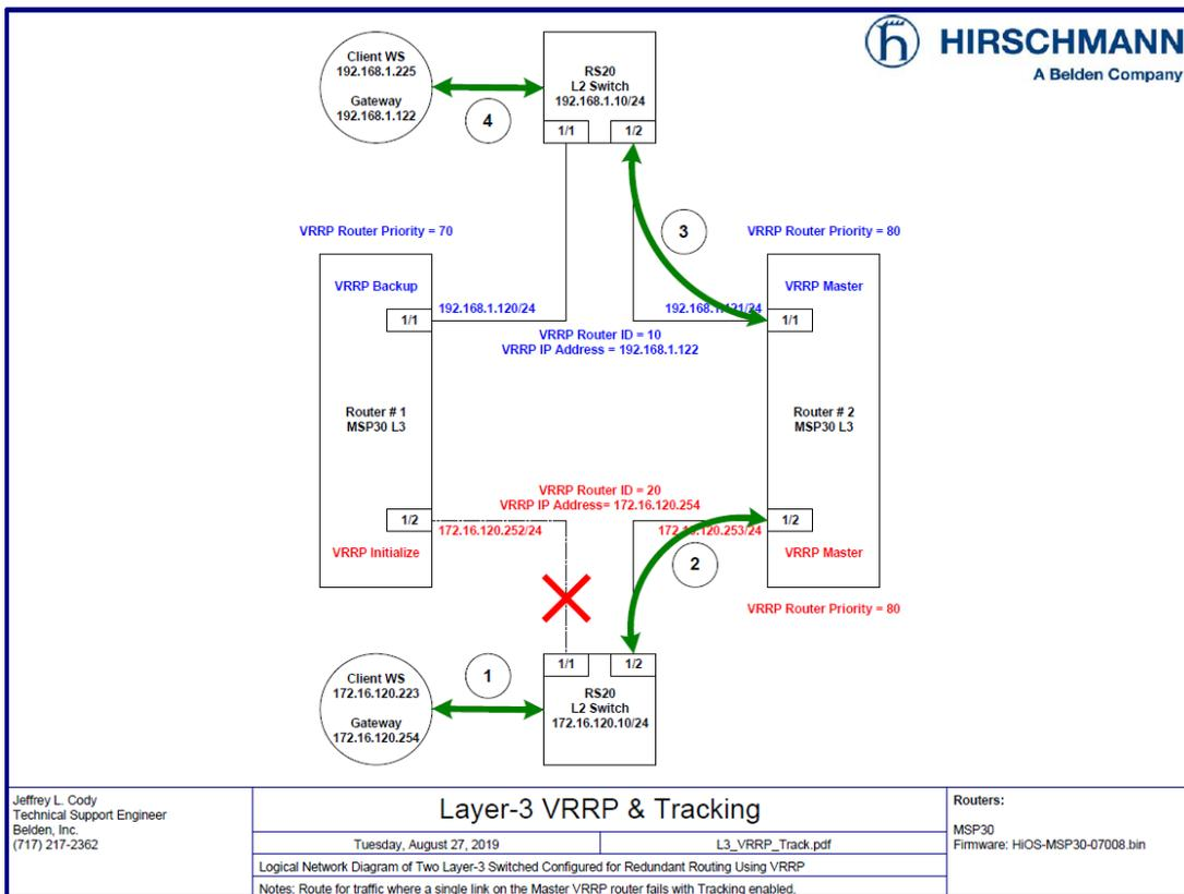
In the diagram above, if we have the same failure of the link between Router # 1 and the L2 switch in the 172 network, and Interface and Ping Tracking is properly configured, we can overcome the previous failure scenario by demoting the VRRP priority on Router # 1 if it senses a failure of the link on port 1/2 by lowering the VRRP priority to 70 for the VRRP router ID 10 on the 192 network.
