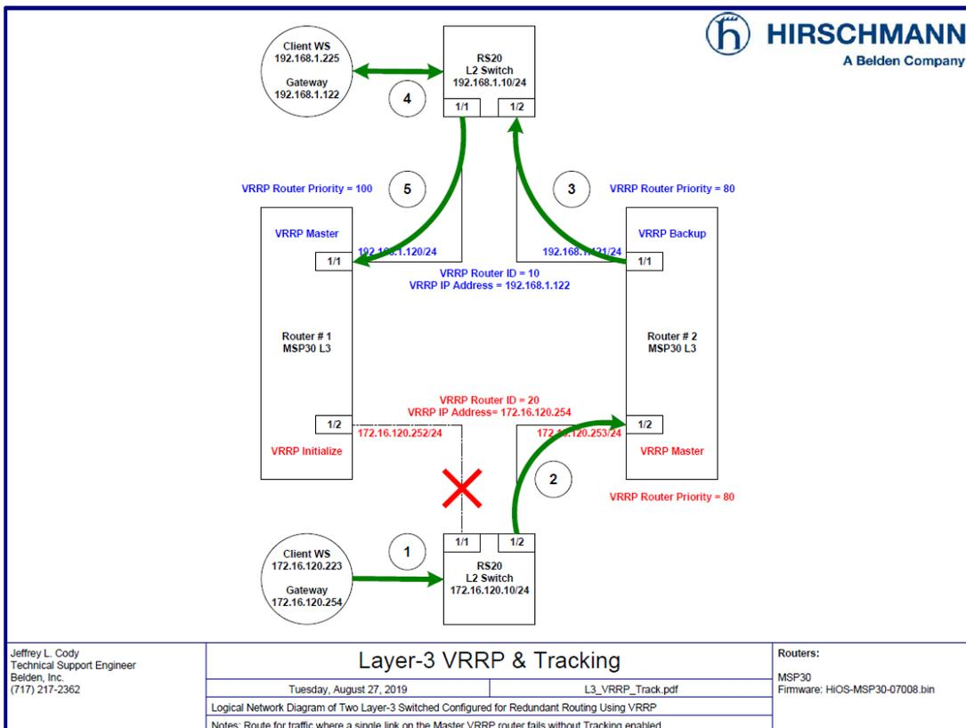
In the diagram above, if we have a failure of the link between Router # 1 and the L2 switch in the 172 network, without Tracking configured, we can have a scenario routing between the two Client WS' will fail.
