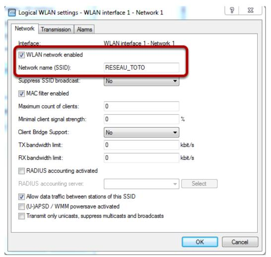
Enable the WLAN network and enter the desired SSID. In our example: RESEAU\_TOTO
