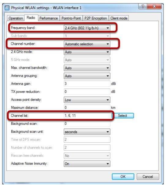
Configuration > Wireless LAN > General > Physical WLAN settings > WLAN interface 1 > Radio tab
