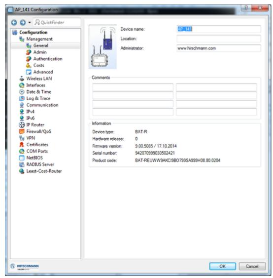
You can open the configuration dialog selecting the device > right clic > configure
