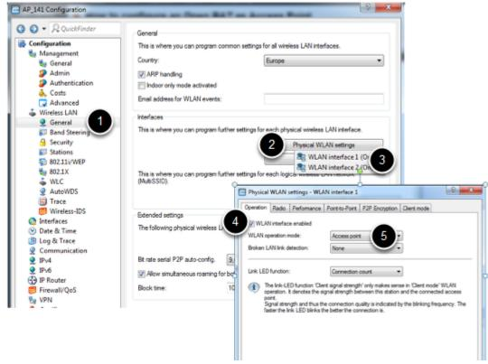
Configuration > Wireless LAN > General > Physical WLAN settings > WLAN interface 1 > tick ""WLAN interface enabled""
