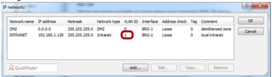
To make the BAT reachable from a VLAN assign the network INTRANET to a specific VLAN. Configuration > IPv4 > General > IP networks
