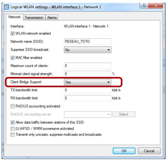
The Client Bridge Support must be enabled.
