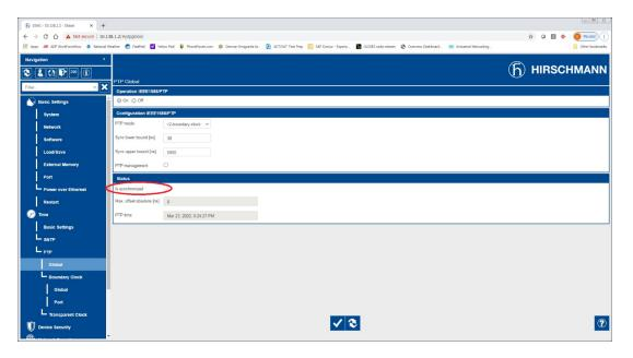
Next browse to Time->PTP->Boundary Clock->Global. Here you should be able to see the Priority 1 and 2 values under Grandmaster match the 127 set in the PLC Date/Time settings. The Grandmaster Identity should be the MAC address of the PLC EN2T card with "ff fe"
