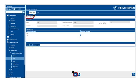
Navigate to the FLM dialog (Network Security - Packet Filter - Routed Firewall Mode - FLM)
