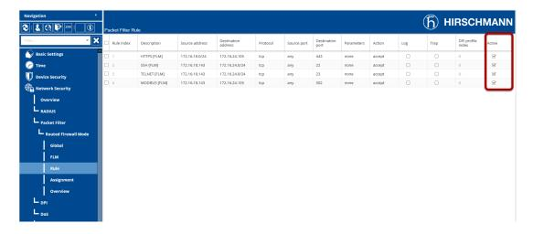
Navigate to Network Security - Packet Filter - Routed Firewall Mode - Rules to check the created rules.
