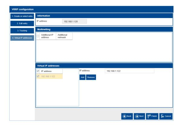
We then repeat the same steps to configure the VRRP configuration for the router interface configured on Port 1/2.
