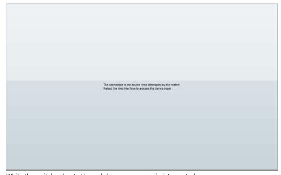
While the switch reboots the web browser session is interrupted. Reload the web interface after the switch completely booted up. Depending on the used hardware this can take up to 2 minutes.
