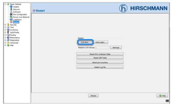
To activate the new uploaded firmware a "Cold Start" needs to be performed.
