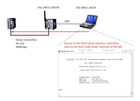
In this example we'll use the COM Port server function of the BAT to access the serial interface of a RS20.
