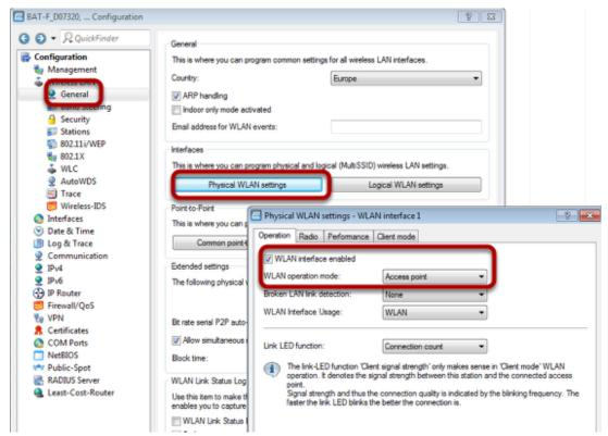
Use Access-Point as WLAN operation mode. Optionally you can choose alternative Radio settings etc.
