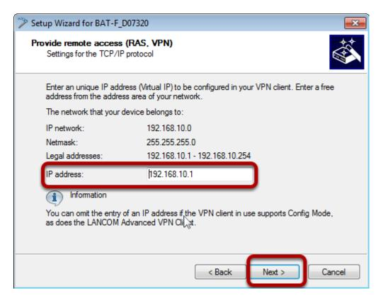
Choose a virtual IP address for the remote client in the local network. This will use proxy ARP automatically.
