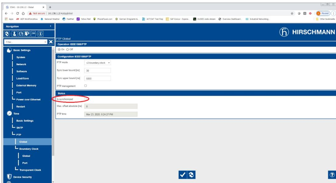
Next browse to Time->PTP->Boundary Clock->Global. Here you should be able to see the Priority 1 and 2 values under Grandmaster match the 127 set in the PLC Date/Time settings. The Grandmaster Identity should be the MAC address of the PLC EN2T card with “ff fe”
