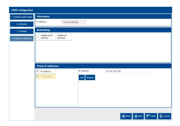
Back on the VRRP Configuration page, ensure that both of the entries are Active. If they are not click the Load button ( $\stackrel{\triangleright}{\square}$ ). If they still are not Active, then click the Active check boxes for each of the VRRP entries, and then click Write button ( $\stackrel{\checkmark}{\square}$ ) at the bottom of the page.
