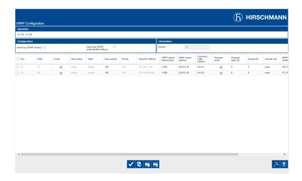
You should now see both of the VRRP instances configured on this router are Active, and the state of each instance is Master. You may need to click the Load button ( one final time.
