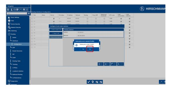
The newly created VLAN-Based Router Interface will appear in the Routing – Interfaces – Configuration page of the GUI as Port vlan/16.
