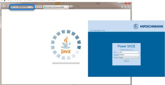
Open your web browser and type the ip address of the switch into the address field of the browser.
