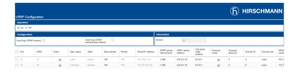
On Router # 2's Routing - L3-Redundancy - VRRP - Configuration page of the GUI, click the Reload button ( ). Notice that port 1/2 is in the Master state.
