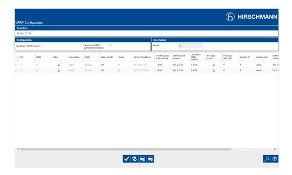
You should now see both of the VRRP instances configured on this router are Active, and the state of each instance is Backup. You may need to click the Load button ( ) one final time.
