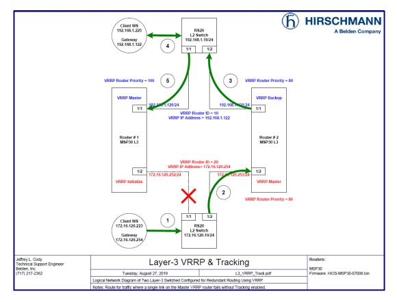
In the diagram above, if we have a failure of the link between Router # 1 and the L2 switch in the 172 network, without Tracking configured, we can have a scenario routing between the two Client WS' will fail.
