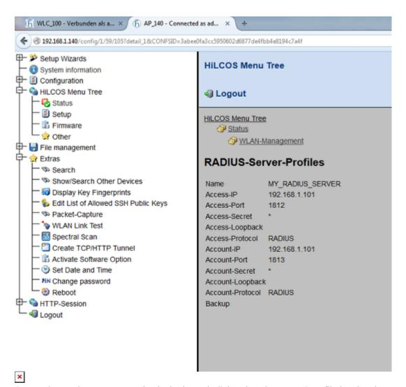
Connecting to the AP you can check via the web dialog that the RADIUS Profile is taken in account under:
