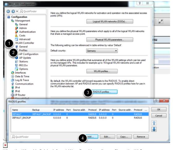
When the Wizard is finished, from LANconfig add a radius profile on the WLC.
