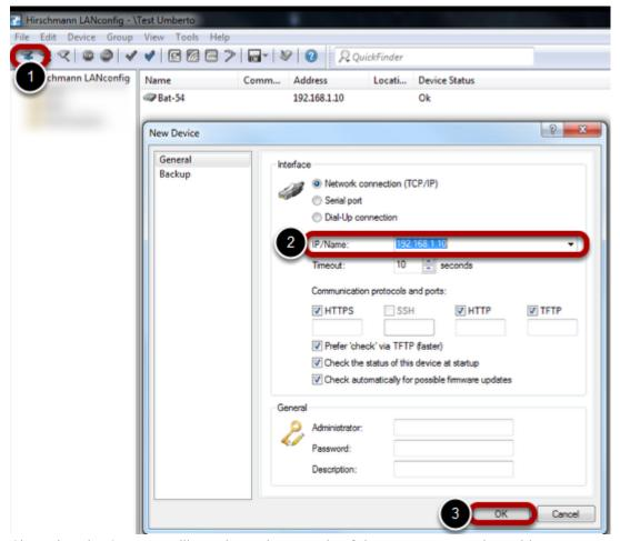
Given that the OpenBat will now have the same ip of the Bat54, we need to add a new device using such ip: 192.168.1.10
