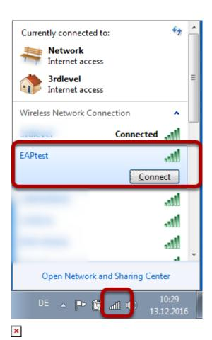
Click on the WLAN icon in the taskbar and choose the relevant WLAN (EAPtest) to connect to.
