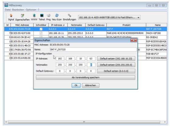
Use HiDiscovery to assign a IP-address to the BAT. The PC is locally connected.
