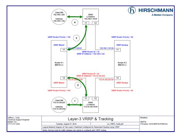
This drawing shown the normal traffic route that is used when the Client WS in the 172 network pings the Client WS in the 192 network when Router # 1 is functioning as the VRRP master router.
