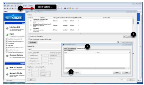
From Wireshark main Windows, open the Capture Options window (Capture/Options...). Clic on manage Interface and select the tab Remote Interfaces and clic on Add
