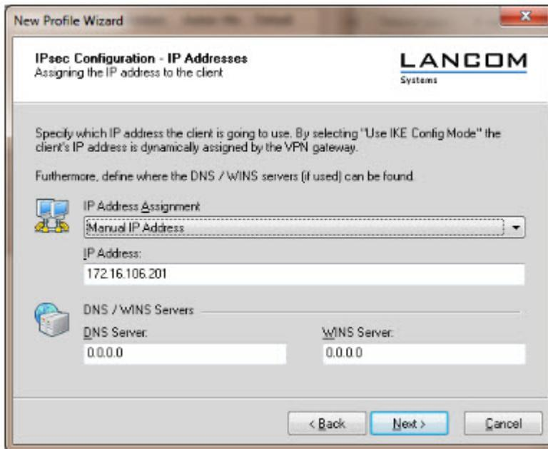
Set the **IP Address Assignment** to **Manual IP Address**.
