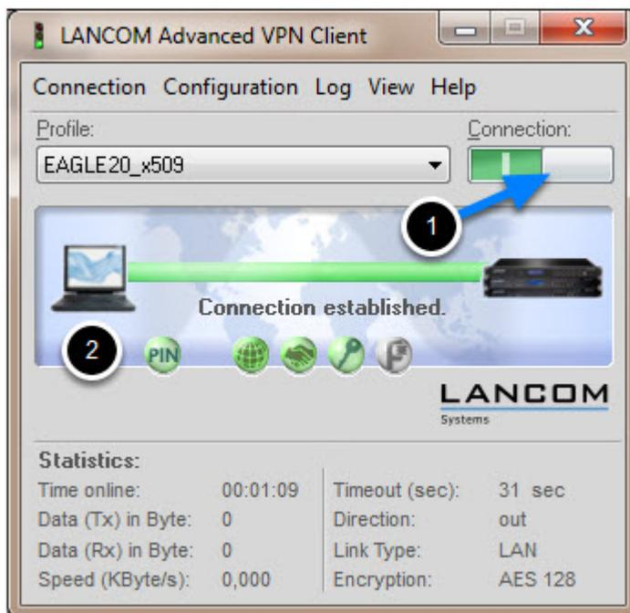
1. Move the Connection slide to the right to initialize the tunnel setup. You will get prompted to enter the certificate's pin. In our example 'test'
