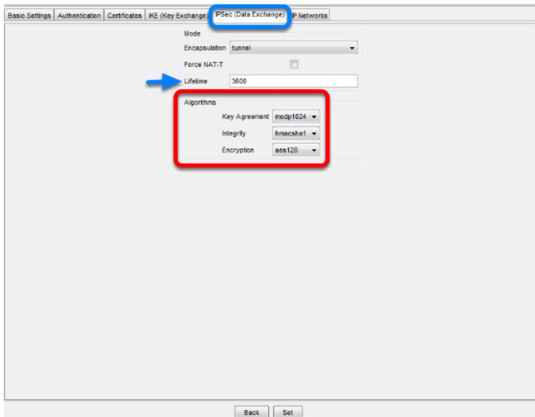
The **Lifetime** in seconds should correspond with the settings of the LANCOM Client (1 hour)
