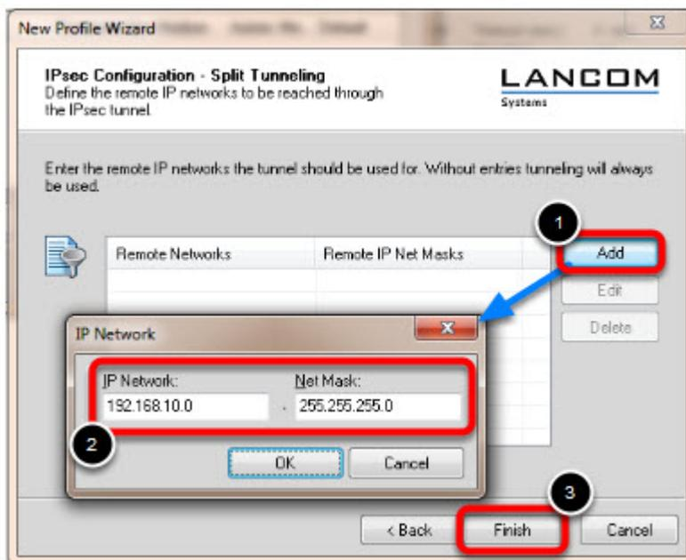
Define the remote IP network to be reached through the IPsec tunnel.
