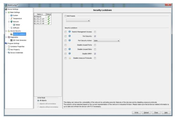
With the Security Lock down dialog you can disable unsecure protocols on multiple devices at the push of a button. evices at the push of a button.
