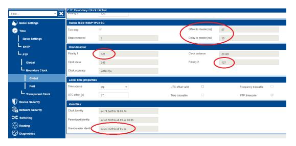
Finally browse to Time->PTP->Boundary Clock->Port. This screenshot shows an install where the PLC is connected to port 6 and the drive(s) are connected to port 4. The PTP status for the PLC port will be shown as "slave" as the switch is a PTP slave to the PLC. The drive(s) will be shown as "master" as the switch relays the PTP traffic from the PLC, becoming the master to the drive(s).
