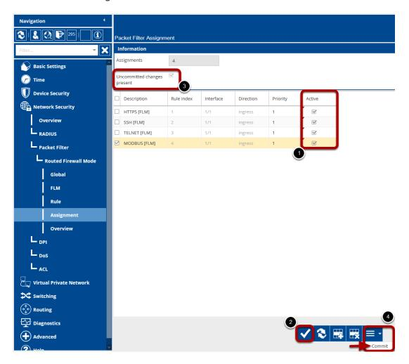
Navigate to Network Security - Packet Filter - Routed Firewall Mode - Assignment to check the interface assignment of the rules.
