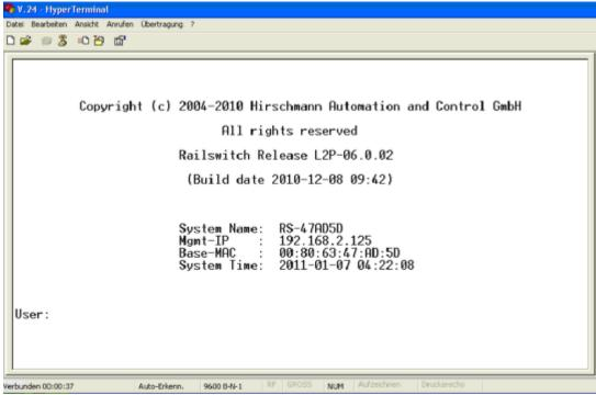
Establish a serial connection to the switch using the terminal cable and a terminal application like HyperTerminal, Tera Term or similar.
