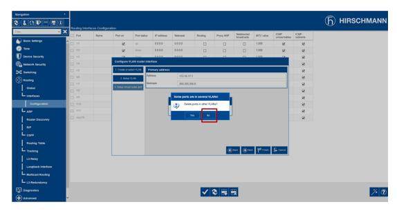
The newly created VLAN-Based Router Interface will appear in the Routing - Interfaces - Configuration page of the GUI as Port vlan/17.
