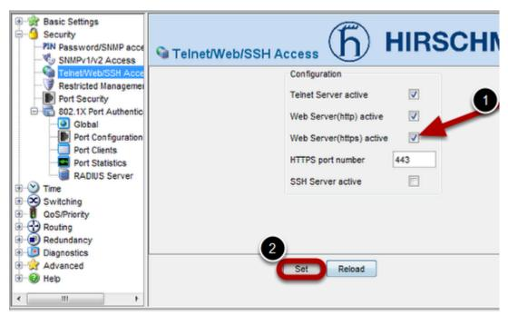
It is necessary to enable HTTPS in order to use radius for access switch agent via WEB-interface.
