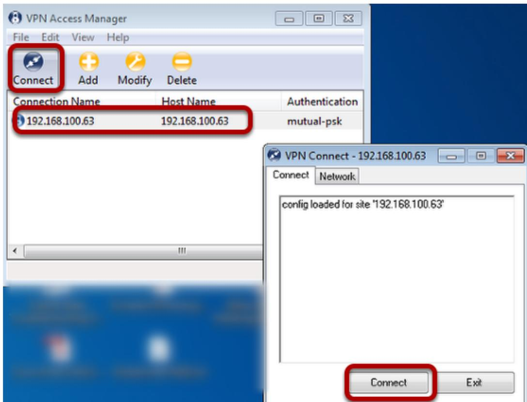
Mark the new created Vpn and press "Connect". A new window will open.
