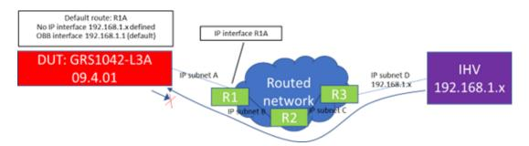
The GRS was configured correctly with a default route pointing to the next interface of router R1. Default IP address is configured for the OOB interface (192.168.1.1) and no changes were made for this interface.
