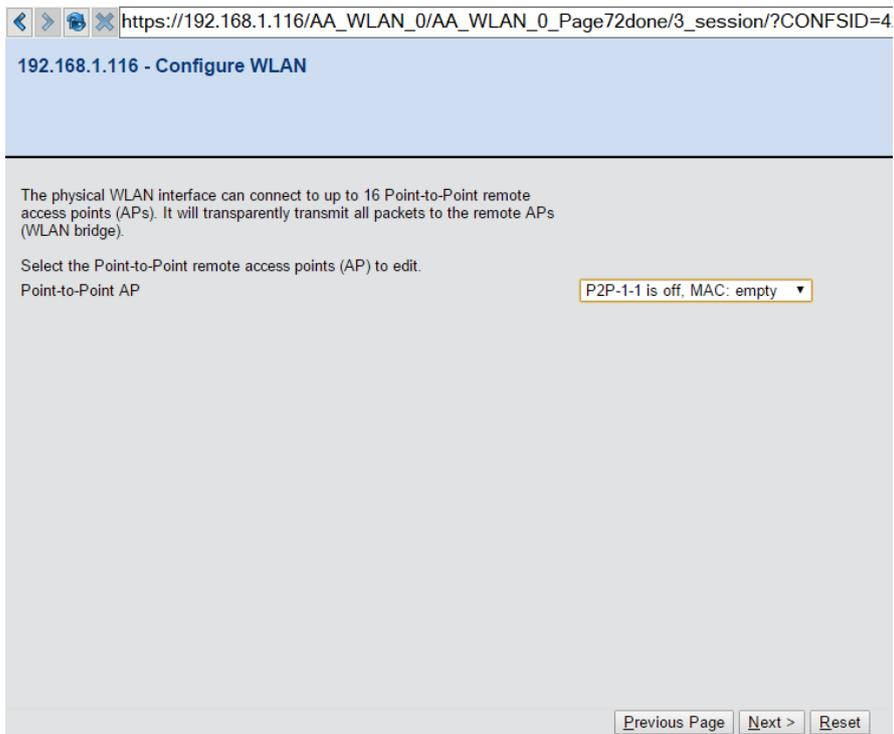
16. Enable the P2P channel, select P2P radio ID of remote site and specify the remote site radio ID, and then click next
