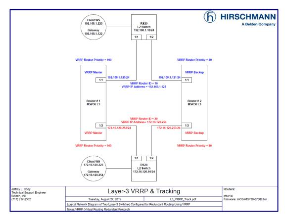
In the diagram above, we see a common VRRP configuration between two routers, Router # 1 and Router #2.
