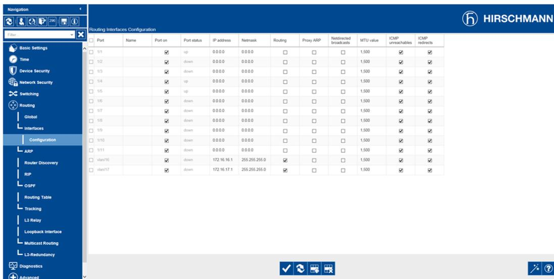
This completes the steps required to configure VLAN-Based (Virtual) Router Interfaces for Ports 1/4 and 1/5.
