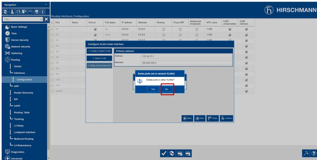
The newly created VLAN-Based Router Interface will appear in the Routing - Interfaces - Configuration page of the GUI as Port vlan/17.
