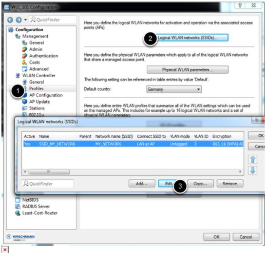
Configuration > WLAN Controller > Profiles > Logical WLAN networks (SSIDs)
