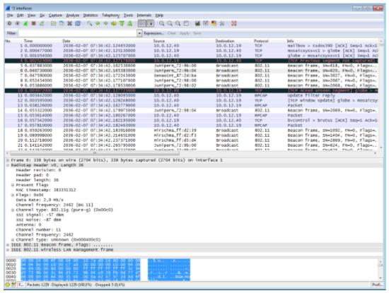
RPCap tunnels the trafic between the BAT and the capturing station. Packets from WLAN-1 with radio header and packets from LAN-1 are in the same capture but can be read separately filtering the interface id.
