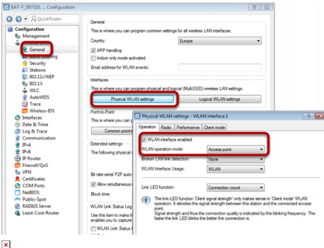
Use Access-Point as WLAN operation mode. Optionally you can choose alternative Radio settings etc.
